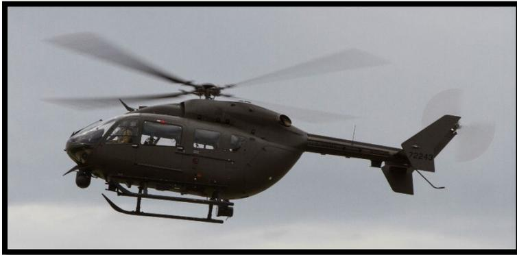
The UH-72A/B Light Utility Helicopter is a Commercial/Non-Developmental-Item, twin engine helicopter with seating for two pilots that is capable of transporting up to six passengers. The UH-72A Lakota operates worldwide in permissive environments to meet Homeland Defense and Security, general support, reconnaissance,
