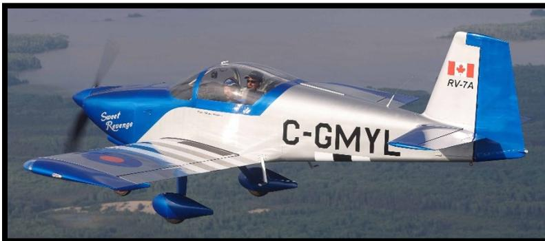
The RV-7/7A retains all the traditional RV virtues. It is an all-around sport airplane, with excellent cross-country capability, fine aerobatic qualities and superior handling. A typical RV-7 can hold two FAA standard pilots, 100 lbs. of baggage and full tanks: 42 gallons. At the
