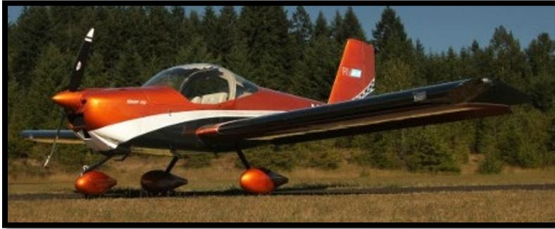
The RV-12 is equipped with a ground-adjustable Sensenich composite propeller — light, smooth and affordable. The light empty weight allows a generous and truly useful load — two 185lb people, a full tank holding 20 gallons of fuel, plus 50lbs of baggage.
