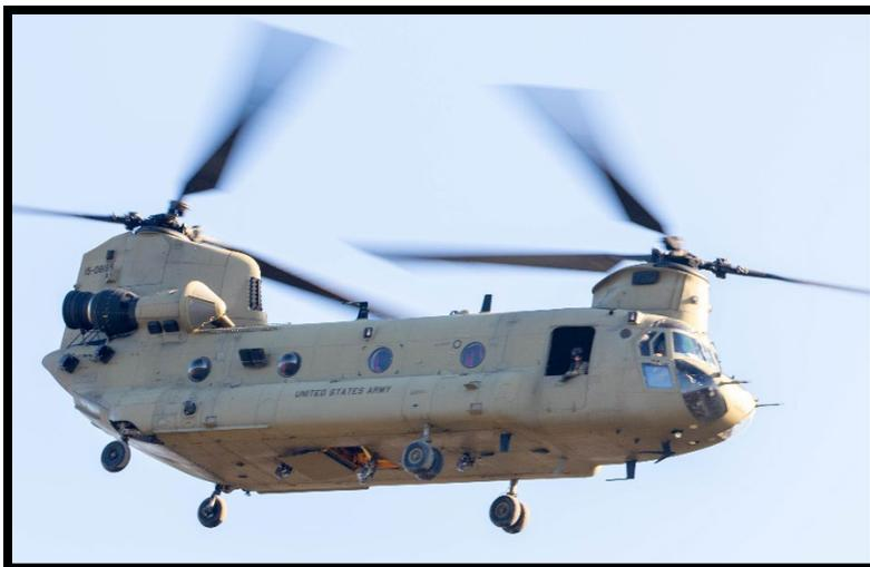
The twin-engine, tandem rotor Chinook helicopter had undergone numerous upgrades since the first CH-47A model was delivered to the Army for use in Vietnam. The Chinook's cockpit accommodates two pilots and an observer. Three machine guns can be mounted on the helicopter, two in the crew door on the starboard side and one window-mounted on the port side.
