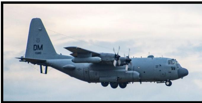
The EC-130H Compass Call is an airborne communications jamming platform. The EC-130 Compass Call aircraft attempts to disrupt enemy command and control communications and limits adversary coordination essential for enemy force management. The Compass Call system employs offensive counter information and electronic attack
