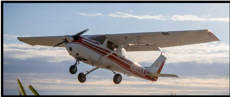
The Cessna 150 is a popular, two-seat, single-engine aircraft designed primarily for flight training and personal use. Known for its reliability, simplicity, and ease of handling, the Cessna 150 is an ideal aircraft for student pilots. With its high-wing design and powered by a 100-horsepower
