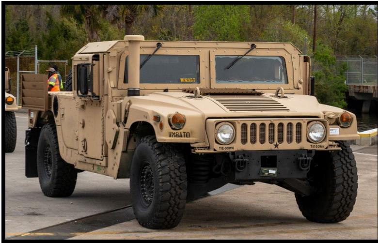
The high-mobility multipurpose wheeled vehicle (HMMWV or Humvee) is a tactical vehicle produced for the US Army. The HMMWV is a lightweight, diesel-powered, four-wheel-drive tactical vehicle built on the M998 chassis common to all its configurations, allowing it to carry military equipment, including machine guns and anti-tank missile launchers.
