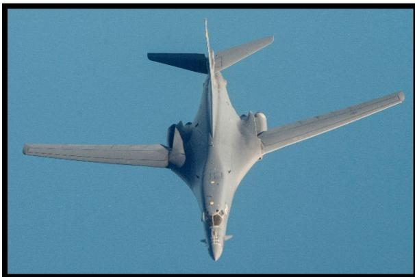
The Rockwell B-1 Lancer is a supersonic variable-sweep wing, heavy bomber used by the United States Air Force. Its 75,000-pound payload is the heaviest of any U.S. bomber. B-1s were primarily reserved for strategic nuclear strike missions at this time, providing the role of airborne nuclear deterrent against the Soviet Union.
