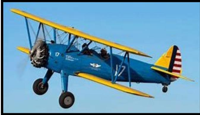
The Stearman (Boeing) Model 75 is an American biplane formerly used as a military trainer aircraft. The U.S. Army Air Forces Model 75 Kaydet had three different designations, PT-13, PT-17 and PT-18, depending on which type of radial engine was installed. It served as a primary trainer for the United States Army Air Forces, the United States Navy throughout World War II. In the immediate postwar years, they became
