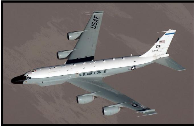
The aircraft is an extremely modified C-135. The Rivet Joint's modifications are primarily related to its on-board sensor suite, which allows the mission crew to detect, identify and geolocate signals throughout the electromagnetic spectrum. The mission crew can then forward gathered information in a variety of formats to a wide range of consumers via Rivet Joint's extensive communications suite.
