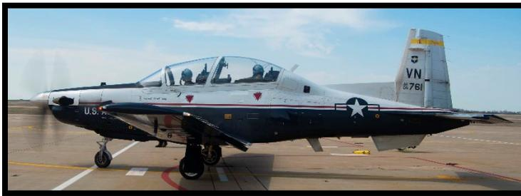
The T-6A Texan II is a single-engine, two-seat primary trainer designed to train Joint Primary Pilot Training Students in basic flying skills common to U.S. Air Force and Navy pilots. Stepped-tandem seating in the single cockpit places one crew member
