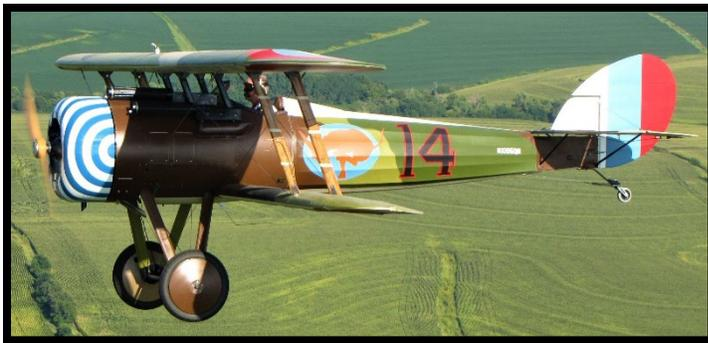
The Nieuport 28 C.1 is a French biplane fighter aircraft flown during World War I. The Nieuport 28 design advanced the concept of the lightly built, highly maneuverable rotary engine fighter. A shortage in 1918 led to Nieuport 28s being issued to four American squadrons, becoming the first aircraft to see operational service with an American fighter
