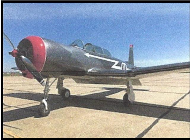
Chuji Jiaolian-6 abbreviated CJ-6 is a two-seat basic trainer and light attack aircraft designed and manufactured in China for the People's Liberation Army Air Force. The CJ-6 can be fitted with two 7.62mm machine guns, bombs, weapons stations and rocket launchers for light attack capability.
