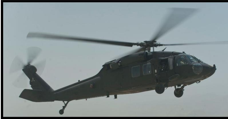
The Black Hawk (UH/HH-60) is the Army's utility tactical transport helicopter. The versatile Black Hawk has enhanced the overall mobility of the Army due to dramatic improvements in troop capacity and cargo lift capability. The Black Hawk provides air assault, general support, aeromedical evacuation, command and
