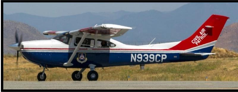
The Cessna 182T Skylane is a four-seat, single-engine, all-metal light airplane. The 182T has fixed landing gear and is powered by a fuel-injected 230-horsepower Lycoming IO-540-AB1A5 piston engine. It is the only variant in production. Civil Air
